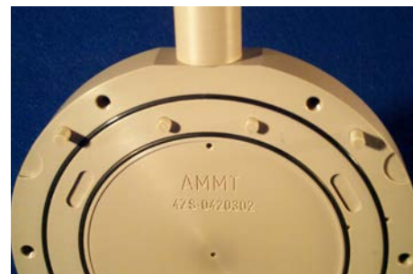
* Wafer holder with enlarge active area option (LAA), the o-ring shape is adapted to wafers flat.
